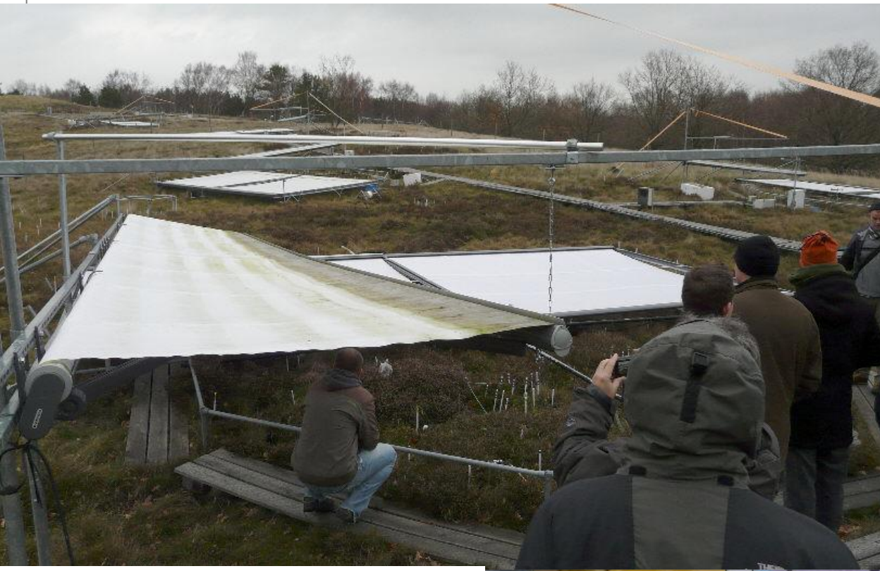
Shielding of precipitation (blind) +ared radiation during the night)
